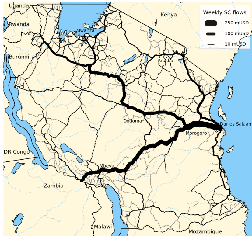
Figure 4-6: Weekly supply-chain flows mapped on the road network. The width of the black lines is proportional to the monetary value of the flow. The widest lines are found on the T1 trunk road connecting Morogoro and Dar es Salaam. It amounts to 224 mUSD per week.
