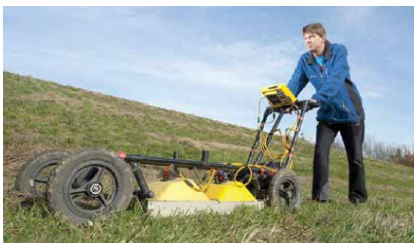
Figure 3: Dam monitoring with use of ground-penetrating radar Picture: AIT
