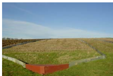
measuring runoff and sediment loss (UK)
