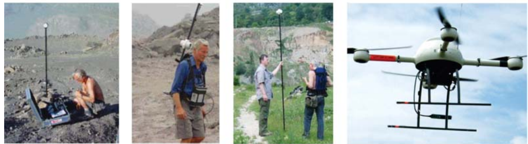
Figure 4.23. From left to right: base station magnetometer, walking mode data collection, sensor height 3 m; UAS.
