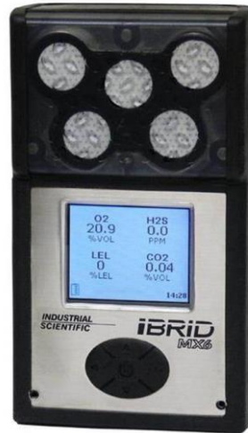
Photo 3.1: Digital CASELLA microdust and 6-gas MX6 iBrid™ meters to be used measure air quality
