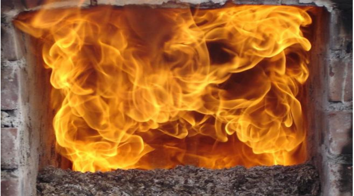
Figure 2: Photo showing Phase-II burning of wood gases (methane) and recycling of the heat gained to push carbonization using Adam retort method
