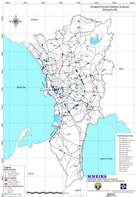
Figure 6.12 Result of Bridges and Flyovers Stability Analysis
