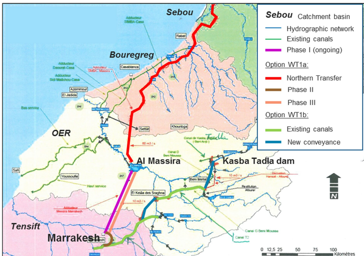
Figure 17 - Outline of the inter-basin water transfer projects to Marrakesh via Al Massira dam or Kasba Tadla dam (source: PDAIRE Tensift)
