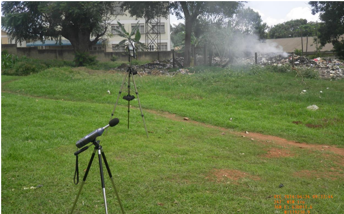
Photo 3.3: Taking noise and air quality measurement behind T.B ward near the proposed site
