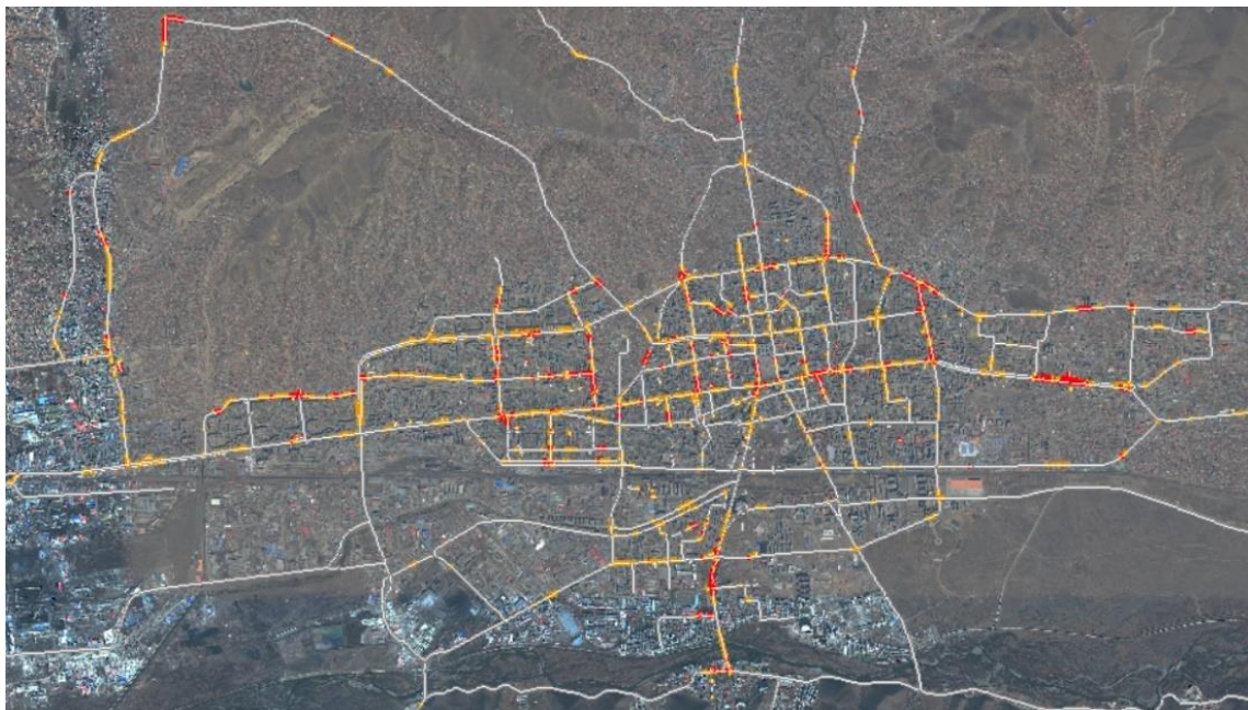
Figure 2.2. High-Priority (red) and Moderate-High Priority (orange) Road Segment for Rehabilitation and Reconfiguration
