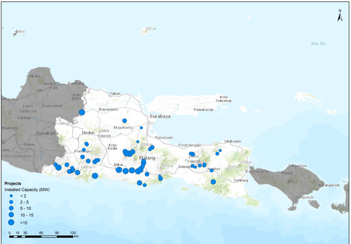
Figure 4.14 – Identified SHP – Distribusi Jawa Timur.
