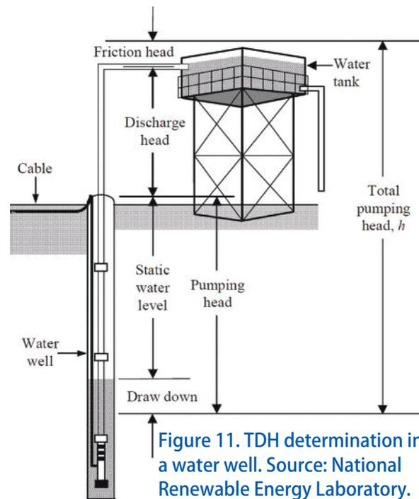
Figure 11. TDH determination in a water well. Source: National Renewable Energy Laboratory.
