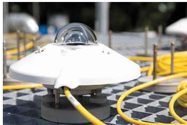
Figure 11: Example Pyranometer Measuring GHI (Image courtesy: Kipp & Zonen)
