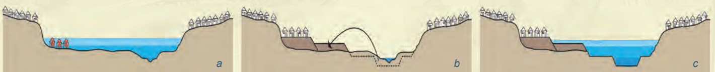
Figure ES-11: Concept of the terraces: At location where currently floods occur (a) cut and fill of dredged material from the river channel capital dredging and maintenance is used to build the terraces (b) with safe locations for new urban areas (c).
