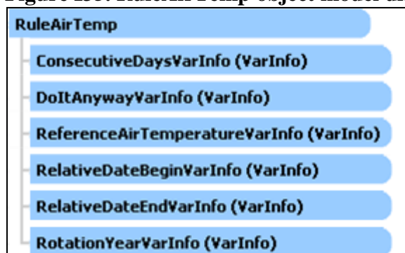
Figure I35. RuleAirTemp object model diagram showing the parameters needed by this rule
