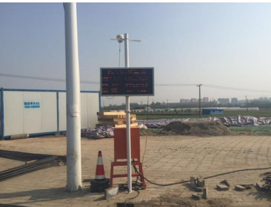
Construction site dust and noise online monitoring system
