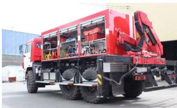
Figure 8.13: Example of HRVs manufactured in Austria and Russia on a commercial truck chassis in 6x4 and 6x6 configuration
