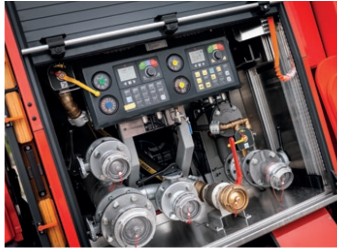
Rosenbauer N110 built-in pump with Hydromatic.
