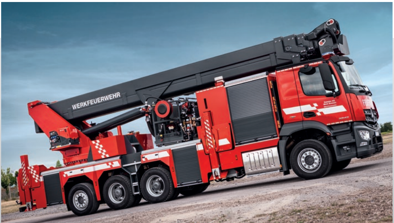
Rosenbauer B51 with N55 pump and Hydromatic foam proportioning.
