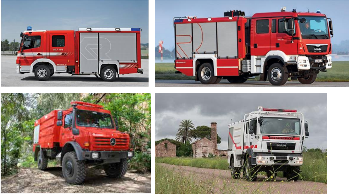
Figure 8.12: Example of ETs of different size and for urban and wildland/mountain environment manufactured in Austria on a Mercedes and MAN truck chassis in 2x4 and 4x4 configuration
