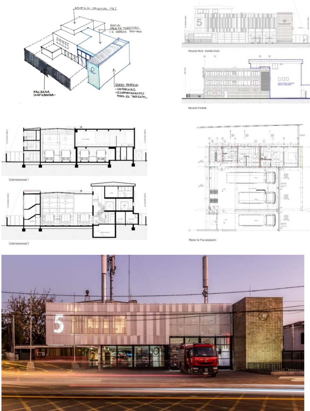
Figure 8.4: Example of area expansion of an existing FRS in Ñuñoa, Chile.
