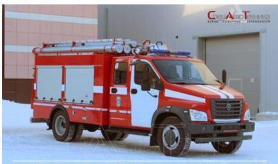
Figure 8.8: Example of BRVs built on a light truck chassis
