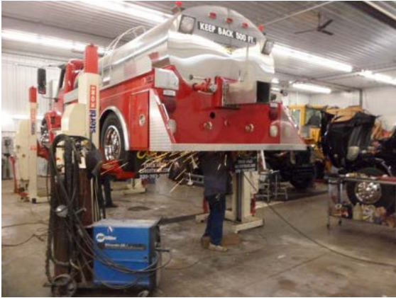
Figure 7.12: Fire apparatus undergoing routine preventative maintenance and servicing [P3].
