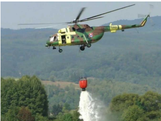
Figure 7.17: Military helicopter using a Bambi bucket on a fire [P3]
