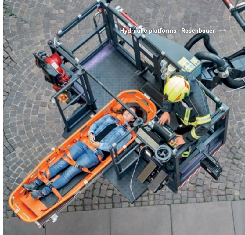
Stretcher storage on the floor for the safe transport of injured persons.
