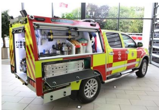
BRV on a Toyota Hilux chassis
