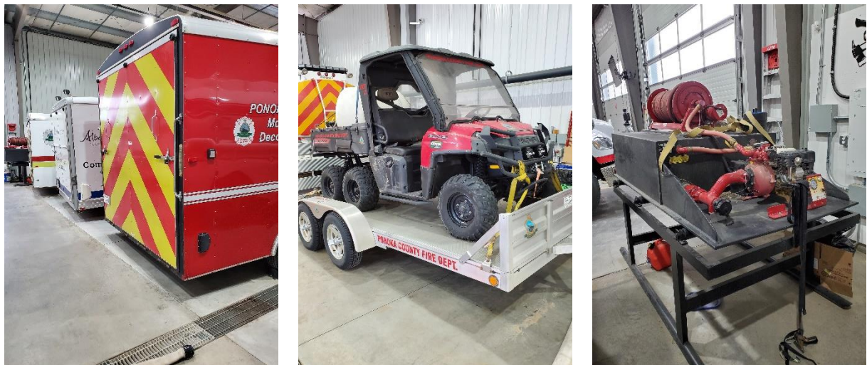
Figure 7.16: Examples for livestock rescue trailers, side by side all terrain unit with small skid tank and pump for remote wildland operations, wildland light truck skid unit (from left to right) [P3]
