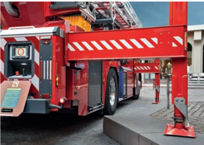
For maximum horizontal reach: the jacking width is continuously adjustable.
