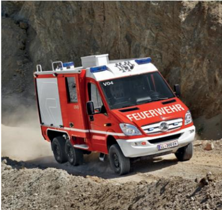
Figure 8.9: Example of special purpose BRVs built on a light truck chassis
