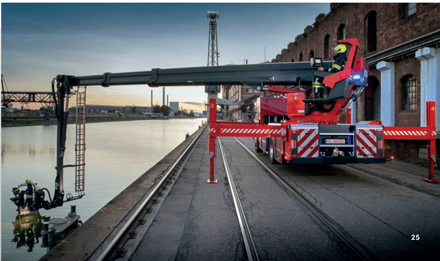
For maximum horizontal reach: the jacking width is continuously adjustable.
