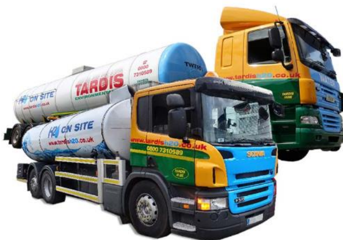
Figure 7.10 Commercial water tankers [P3].
