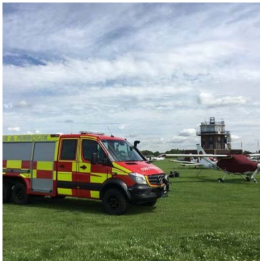
Figure 7.14: Rapid Intervention Vehicle in a 6x6 configuration [P3].
