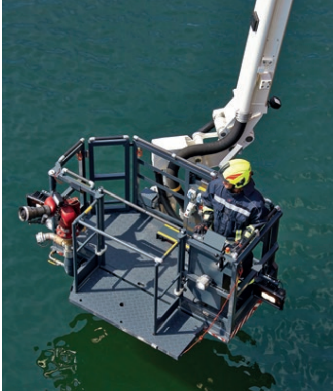
With folding platform, as well as entry options at the front, rear and side.
