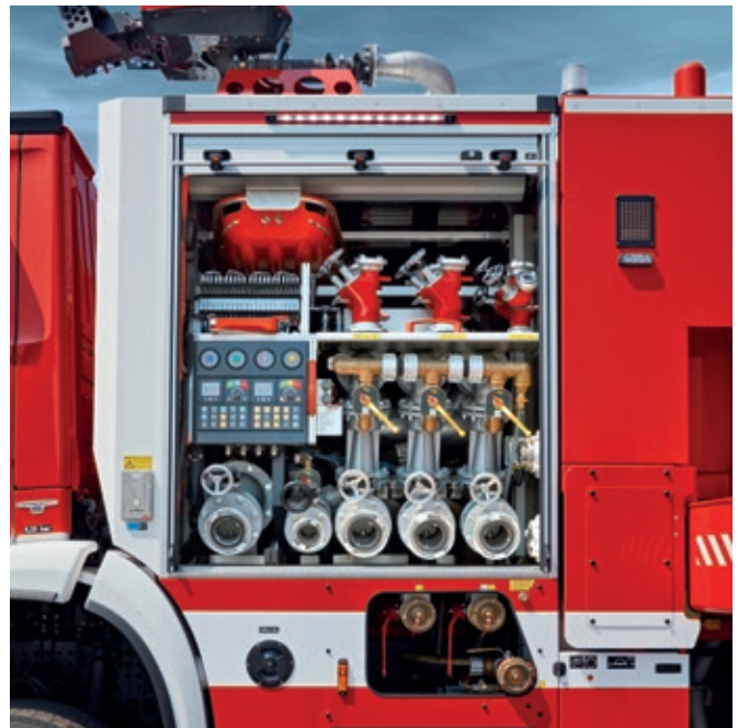
Rosenbauer N80 with Hydromatic foam proportioning in mid-ship installation.
