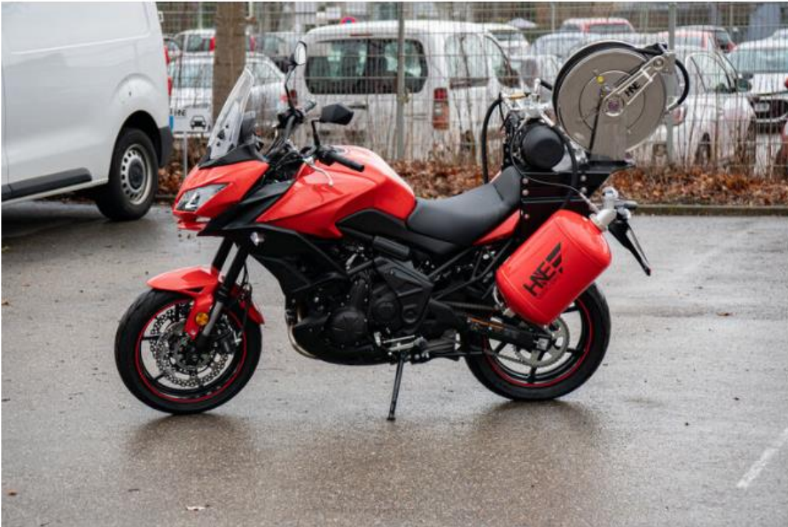
Figure 7.5: Fire bike with CAFS system, [A6]
