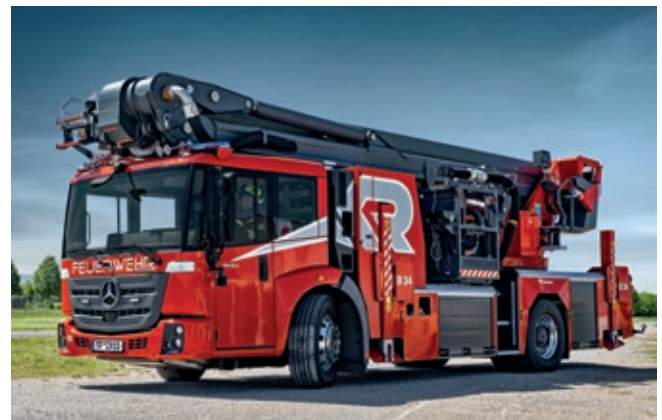
Rosenbauer B34 on 4x2 low floor chassis with just 3.2 m vehicle height.
