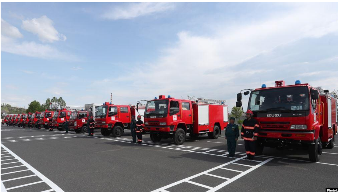
Figure 8.11: Example of ETs manufactured in Japan on a ISUZU truck chassis in 2x4 and 4x4 configuration delivered to Armenia as donation from Japan
