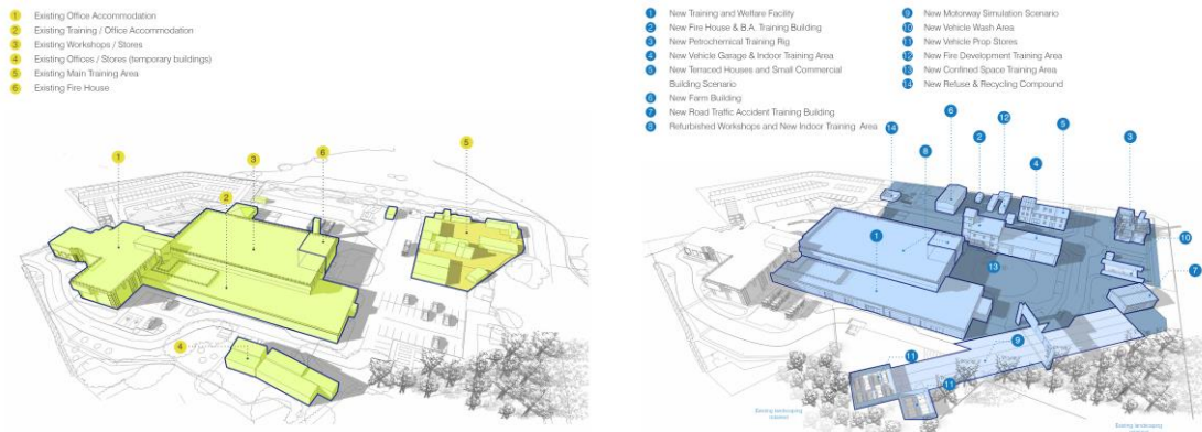
Figure 8.24: Multipurpose training centre developed on existing site reusing some of the existing facilities
