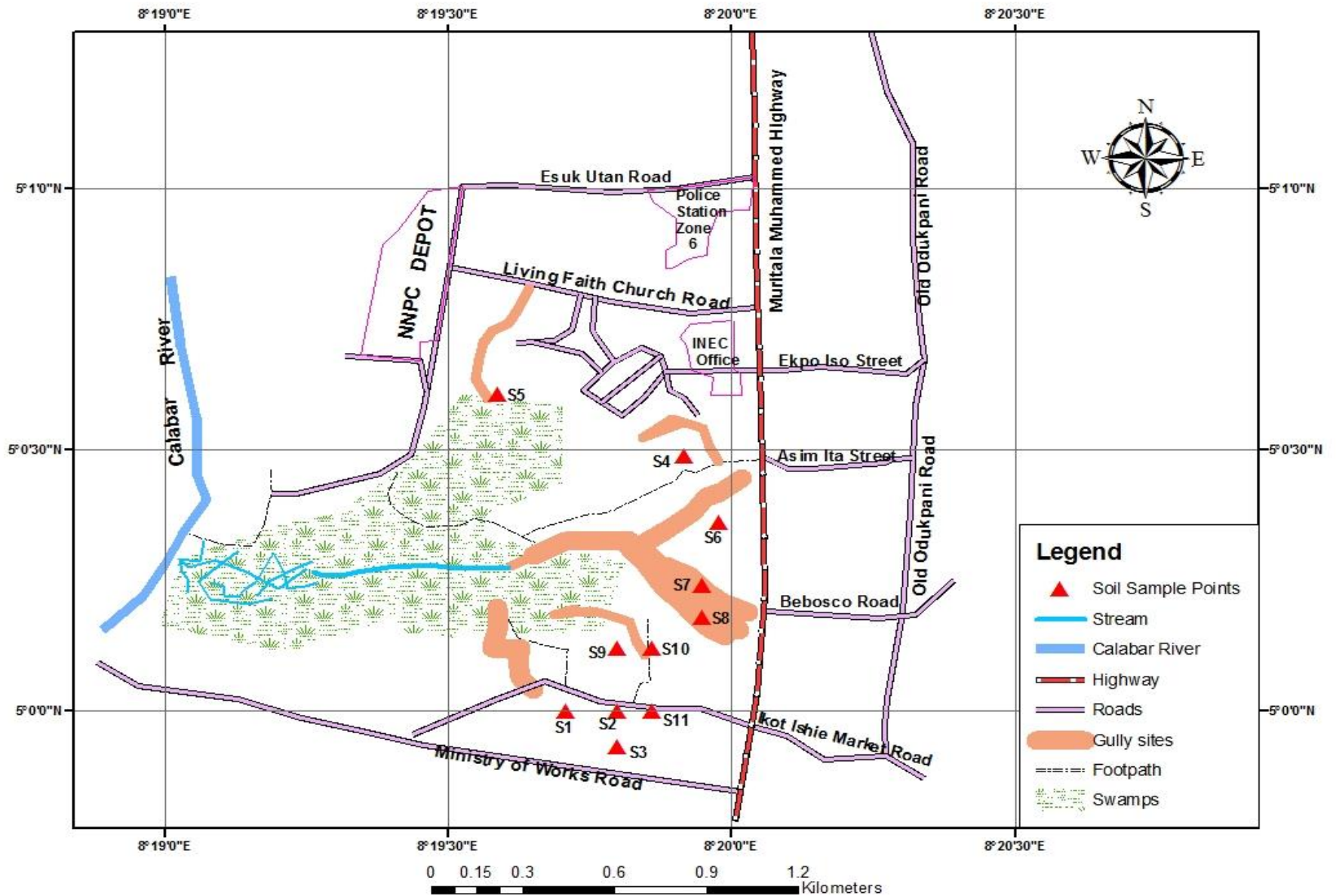
Fig. 3.5: Map Showing Distribution of Soil Sampling Points in the Ikot Anwatim Newmap Project Area
