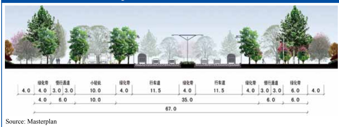
Figure 4.3: Six-Lane Arterial Road
