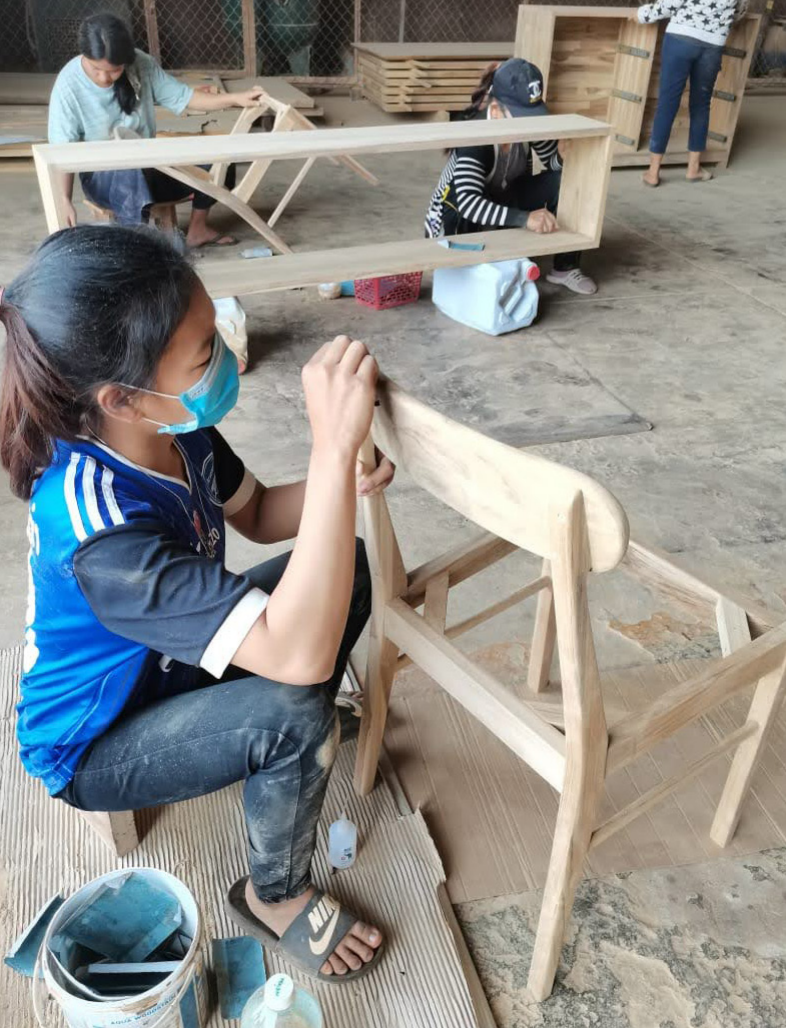
Female daily workers sanding wooden chair frame before painting at wood processing factory, Xaythani district, Vientiane Capital. Photo credit: Dalaphone Sihanath.
