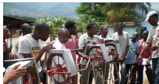
Figure 10: Rope pump manufacture training in Southern Tanzania
