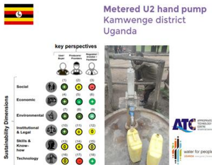
Figure 2: Example summary of a TAF assessment by ATC in Uganda. The traffic light system compares how well the technology fits to context according to 6 sustainability dimensions and 3 perspectives (1. User; 2. Provider/Producer; 3. Regulator/Investor/Facilitator)
