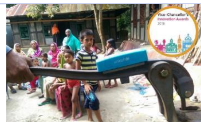
Figure 15: Smart Handpump Sensor fitted to a No.6 Pump in Bangladesh (Photo Courtesy of Oxford University)
