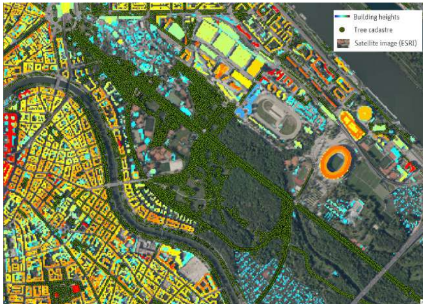
Figure 11. Satellite image and tree cadastre, building footprints, and height layers (using photogrammetry) in the area of the Viennese public park Prater. Source: City of Vienna.
