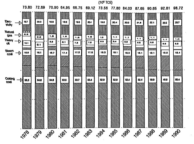
Figure 3.1: PRIMARY ENERGY CONSUMPTION IN THE IRON AND STEEL INDUSTRY, 1990
