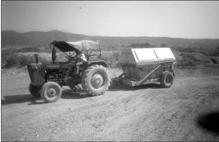
In small towns, containers can be transported by tractors equipped with a container-lifting device.
