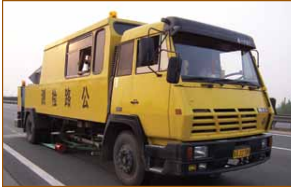
High-Capacity Deflectometer for Deflection Measurements and Pavement Structural Assessment in Hebei Province, China
