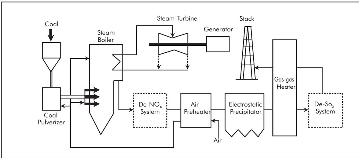
Table 2.17 shows design parameters and operating characteristics for a typical steam-electric power plant. We assume a 300 MW base-loaded plant with a SubCritical boiler.
