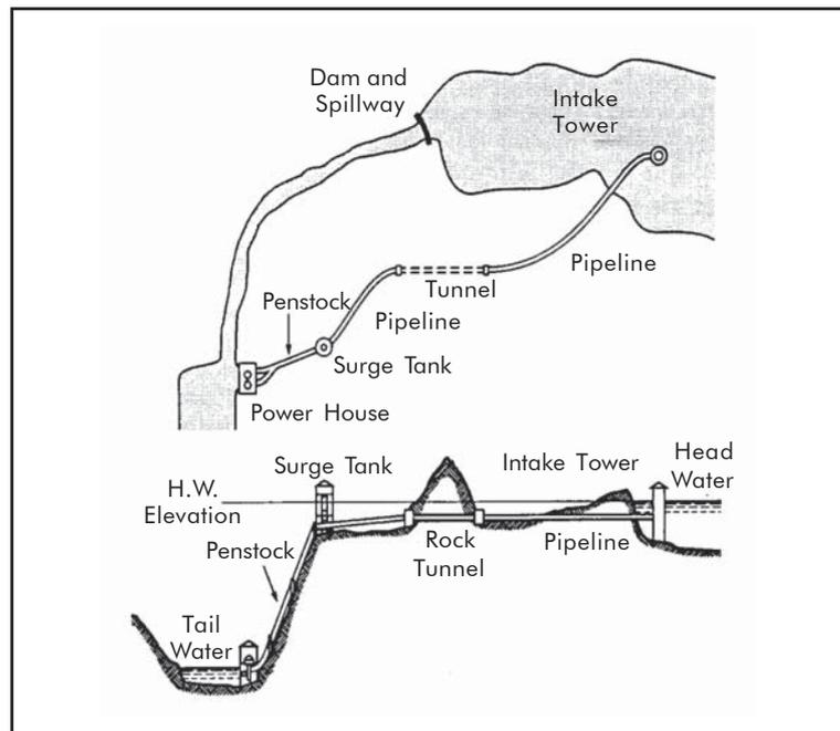
A pumped storage power generation scheme is a specialized scheme in which several power plants are used to optimize the power output in accordance with diurnal variation in system, load. In this scheme the hydroelectric power plant acts both as a generator and a pump, allowing water in a lower reservoir to be pumped up to upper reservoir during the low-load overnight period, and then generating electricity during peak load periods (Figure 2.12).
