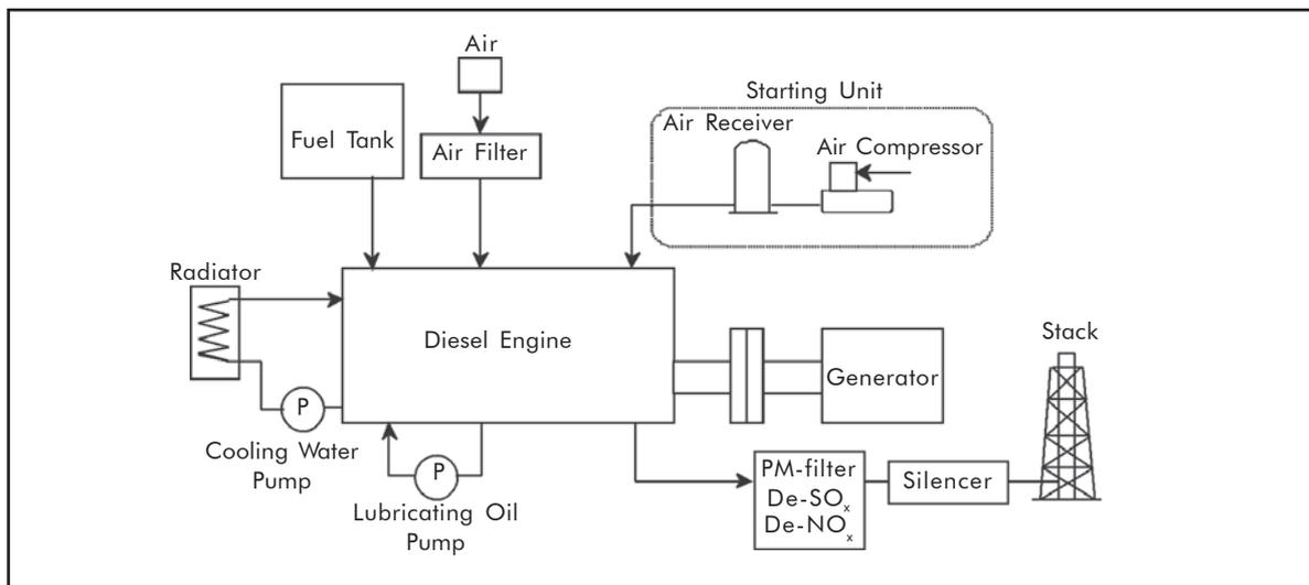
We have chosen four generic gasoline/diesel engine-generator arrangements in order to assess their economic effectiveness across a range of power supply configurations: (i) a 300 W and a 1 kW gasoline engine-generator configured for off-grid use; (ii) a 100 kW diesel engine configured for mini-grid use; and (iii) a 5 MW diesel engine generator
