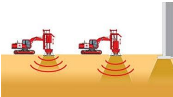
Rapid impact compaction
