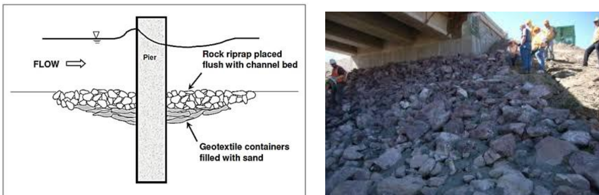
Figure 152. Example of scour mitigation for bridge piers and abutments for wooden bridges
