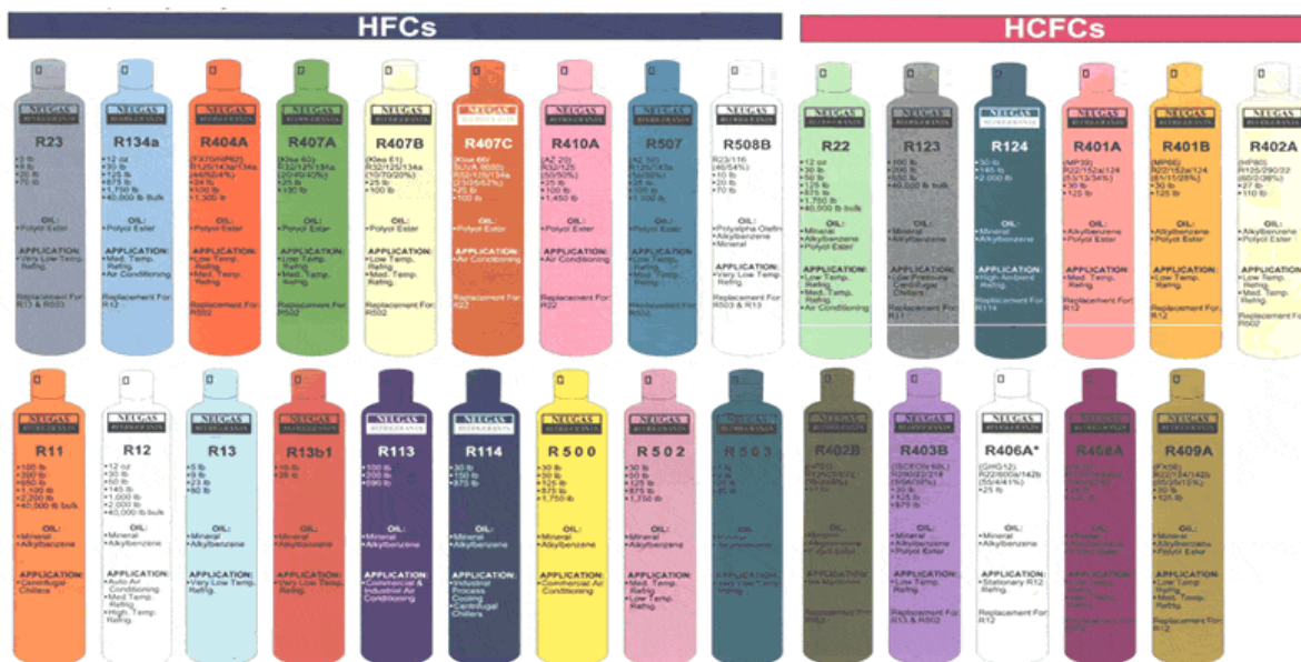
Figure 1 Color Code for Refrigerant container
