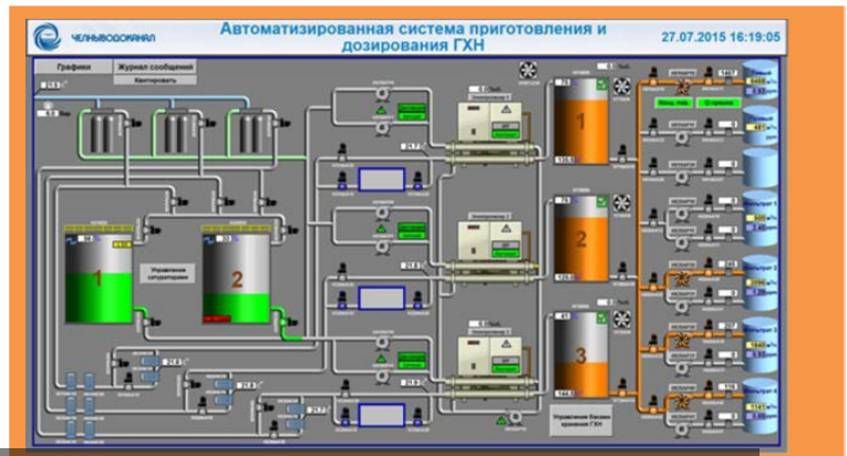
Automatic system of preparation and dosing of 0,8% sodium hypochloride for water disinfection in Naberezhnye Chelny
