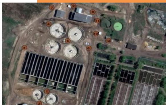
Plan of sewage treatment plants new line in Saransk
