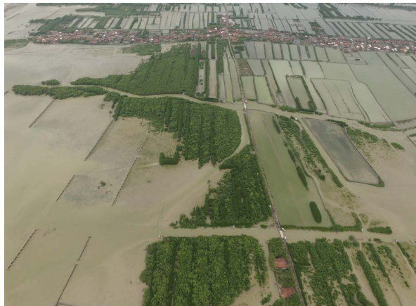
Sediment accumulation behind permeable grids in Demak, Central Java, Indonesia. (Source: Wetlands International)
