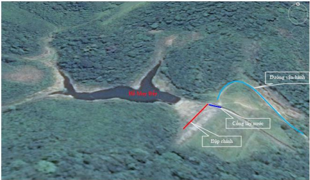
Figure 2: The diagram of works belonging to The May Day reservoir - Dong Xa commune
