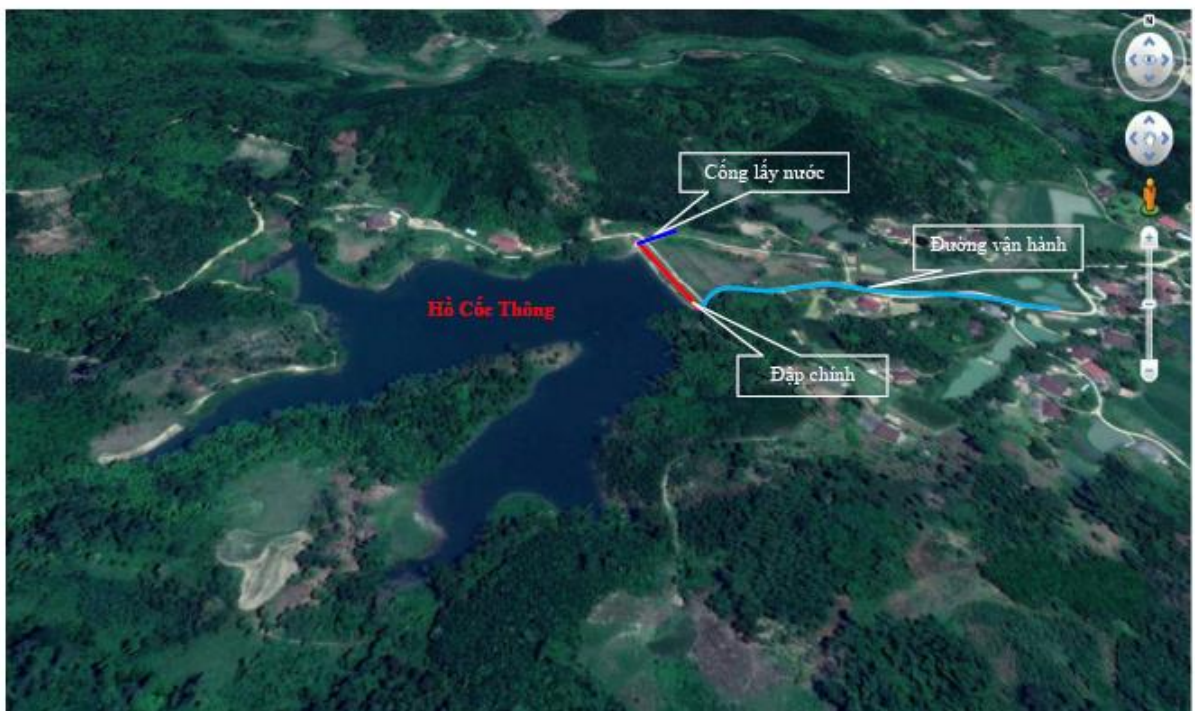
Figure 3: The diagram of works belonging to The Coc Thong reservoir - Liem Thuy commune
