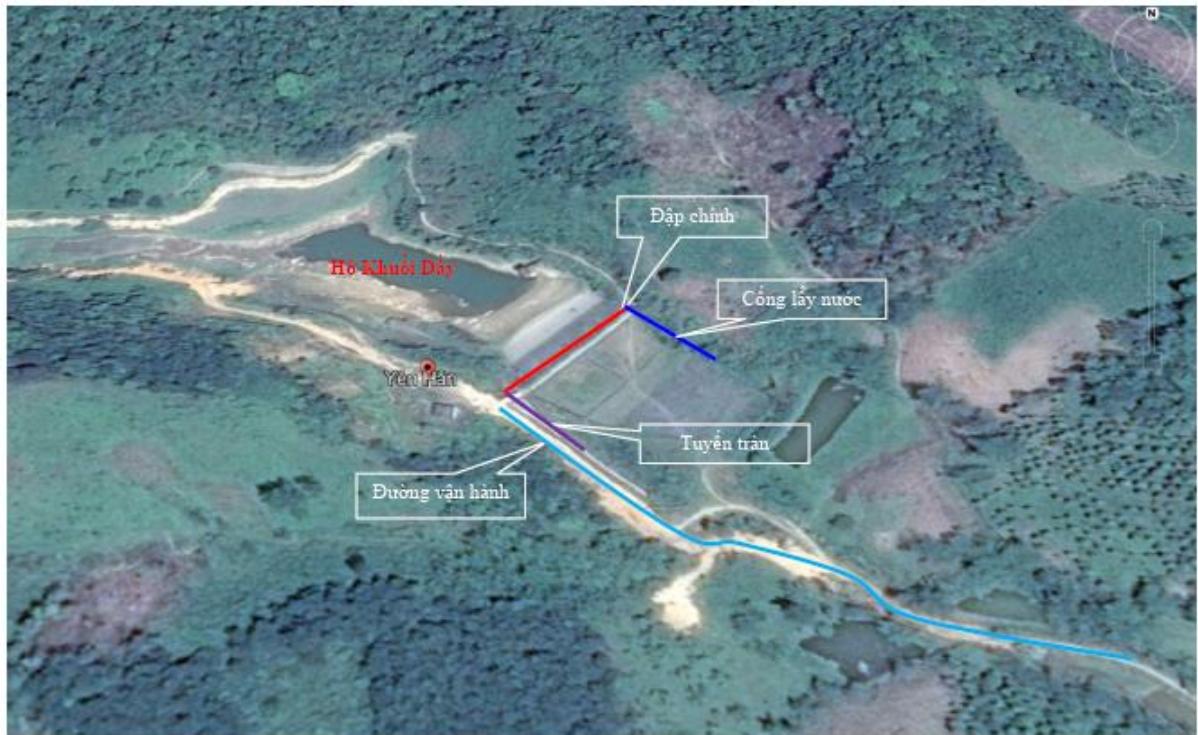
Figure 6: The diagram of works belonging to The Khuoi Day reservoir - Yen Han commune
