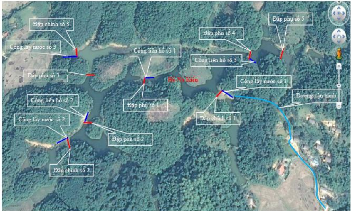
Figure 4: The diagram of works belonging to the Na Kien reservoir - Nghia Ta commune
