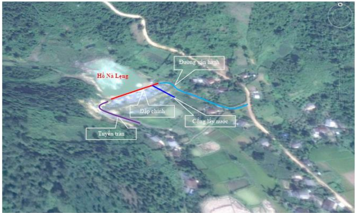
Figure 8: The diagram of works belonging to The Na Leng reservoir - Sy Binh commune
