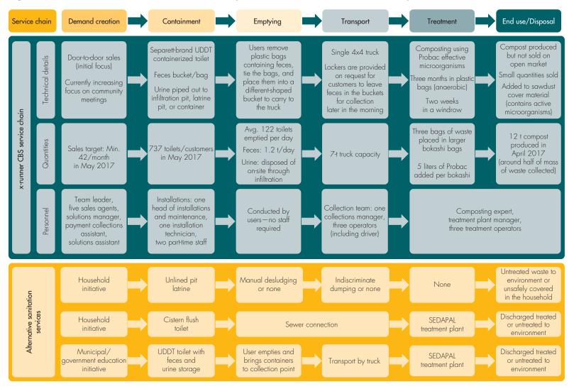
Figure 2.1 • Sanitation Service Chain for Sanitation Options in x-runner Catchment Area (as of April 2017)
