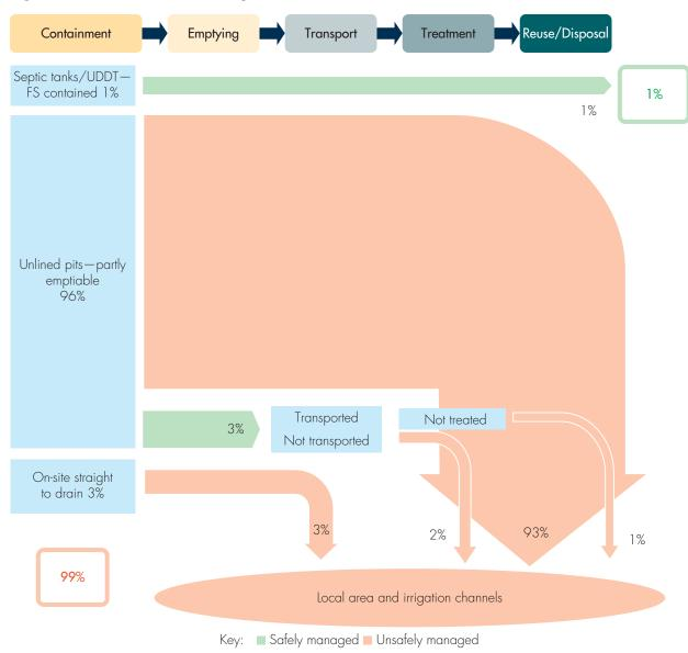
Figure 1.2 • Fecal Waste Flow Diagram for Nonsewered Areas in Lima
