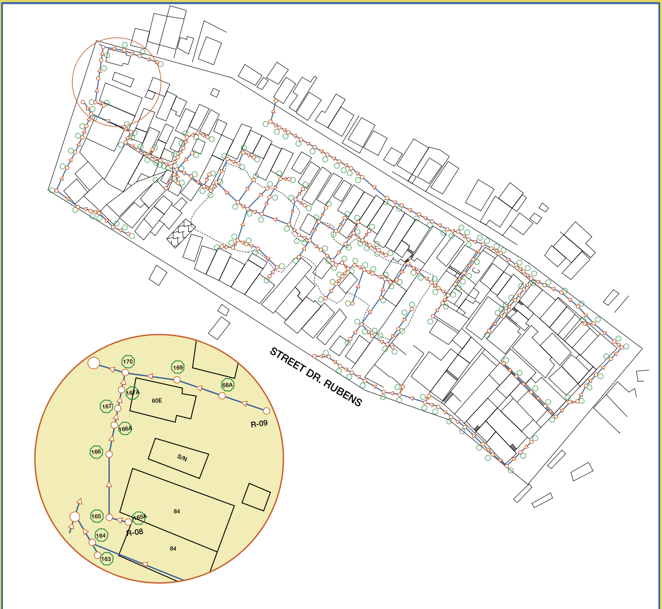
Figure III.5: Illustration of condominial branch design in Bacia do Alto Camajuripe
