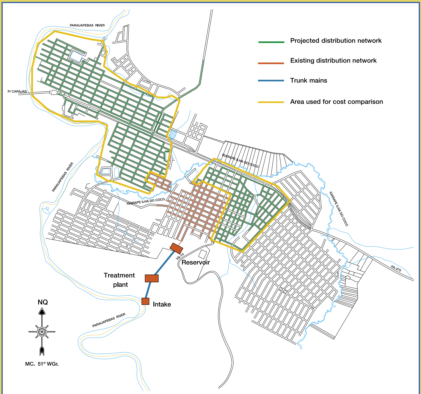
Figure IV.1: Original conventional water system design for Parauapebas
