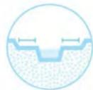
**Riverbanks:** Floodplain restoration often includes reshaping river banks to prevent erosion and support natural vegetation. Such shaping should be accompanied by appropriate bank stabilization and revegetation measures, which typically include the use of an appropriate mix of seeds, and vegetation adapted to soil conditions and tolerant to periodic inundation.
