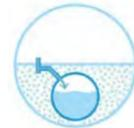
**Hybrid infrastructure:** Bioretention areas can be effectively combined and connected with sewer systems through an overflow outlet or through underdrains that connect to the sewer system. By attenuating runoff, bioretention areas relieve the pressure of runoff and contribute to storm water management—integrating green and gray.
