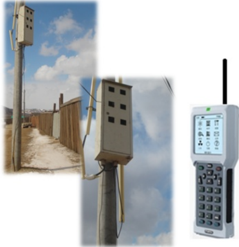
TP900 remote type Hand Held Meter Reading Devices is used to read meters with DDSF22/RF/ type radio modem
