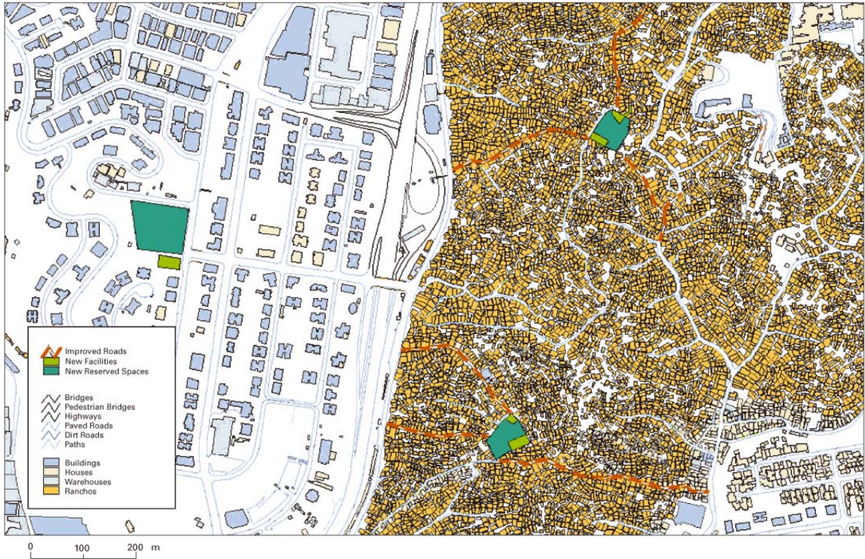
Figure 5.6. Proposed interventions in a section of Petare to improve disaster preparedness with the allocation of reserved space
