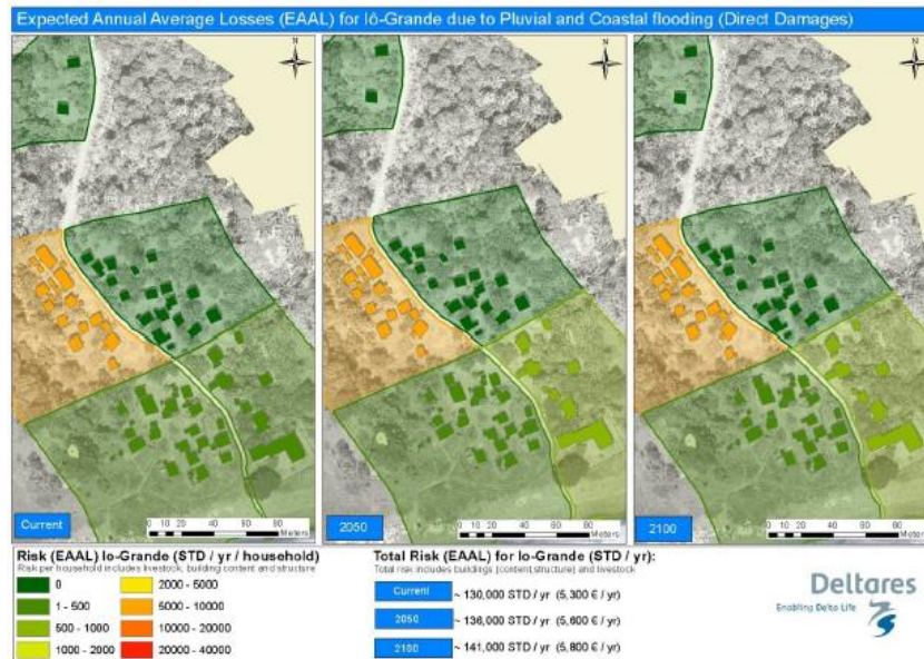
Figure 5.3: Total EAAL and EAAL per household in Iô Grande, due to direct economic damages only, from pluvial and coastal flooding
