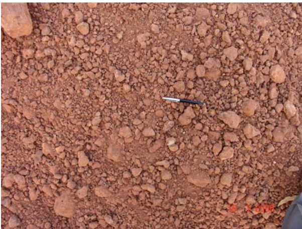
Laterite nodules, when hard enough, can be screened to produce a satisfactory aggregate for a bituminous surfacing
