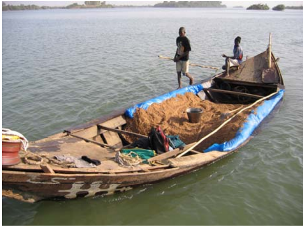
Extraction of gravel from the River Niger – a tedious, time-consuming activity yielding typically about 2 – 3 cubic metres per day
