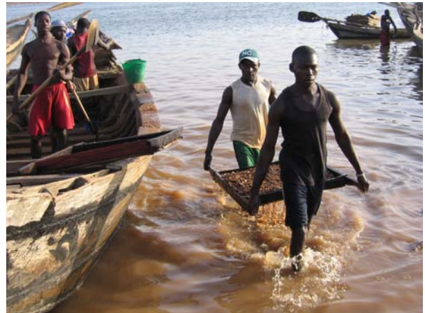
Off-loading and washing of gravel to remove fines prior to stock piling on the river bank
