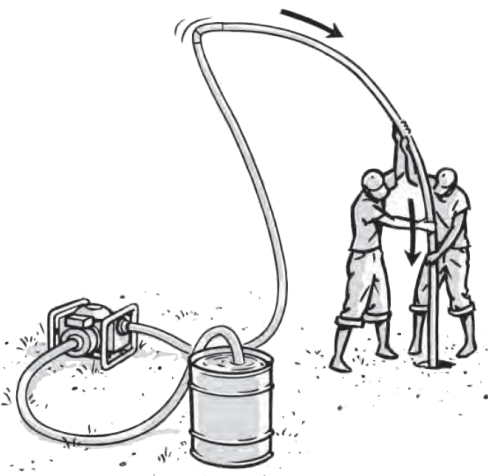
Figure 5: Rapid well jetting
