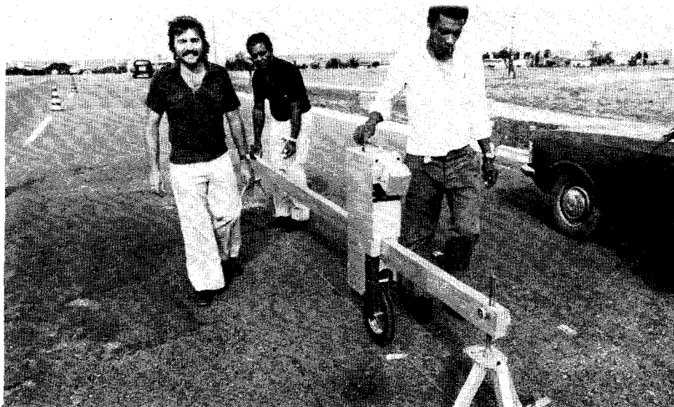
Figure 3. Measurement of longitudinal profile with the TRRL Beam.
