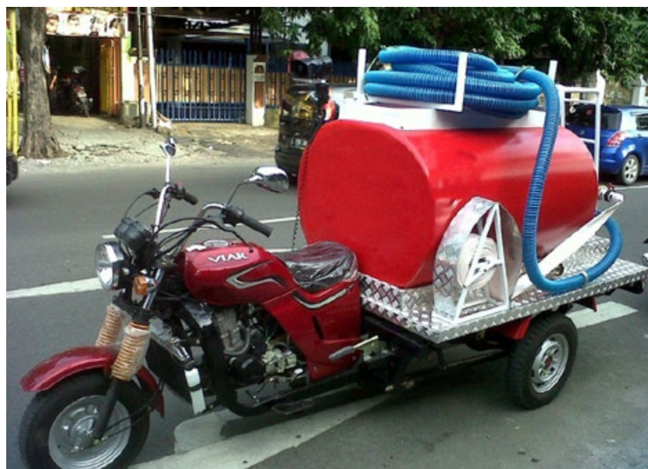
Figure 16. Fire-fighting vehicle which fits narrow roads in dense settlements.
