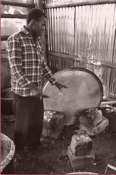
Figure 17. An industrial-sized three-stone fire. This is the baseline set-up for large-scale cooking operations such as those in schools and prisons.
