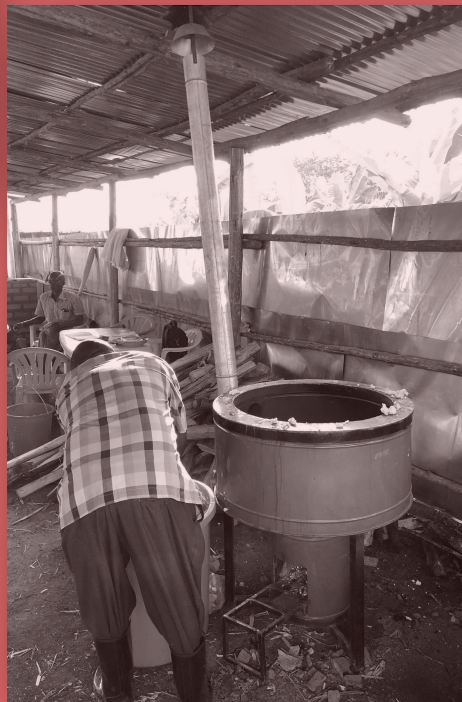
Figure 18. An industrial-sized improved cookstove, which is faster than the baseline three-stone fire, far more efficient, and has the potential to lead to significant savings in the long term.
