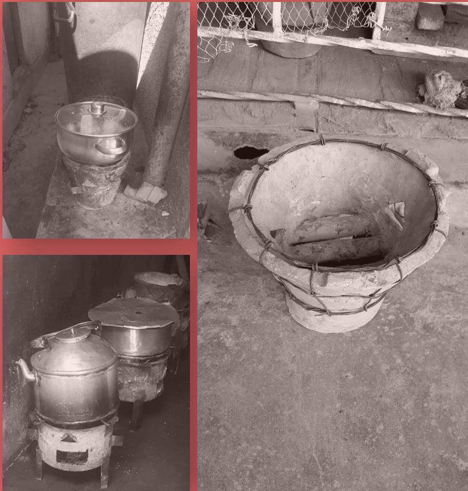
Figure 20. Examples of baseline stoves. Baseline stoves come in a variety of shapes and sizes—purely ceramic, purely metallic, and hybrid ceramic-metal. Typically, they are cheap (under U Sh 3,000), break fairly often (e.g. once every few weeks) and use about twice as much charcoal of an equivalent improved cookstove.
