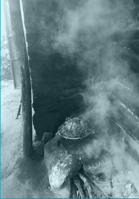
Figure 1. A baseline fire pit located in a peri-urban household. Powered by firewood, this kind of stove is used to cook large meals over a long period of time (e.g., 6–8 hours).
