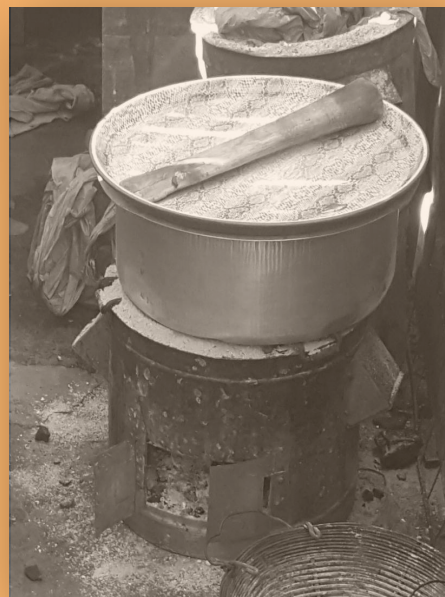
Figure 16. A Ugastove-type cookstove, shown here in operation. This type of stove is the most common we observed during our fieldwork.
