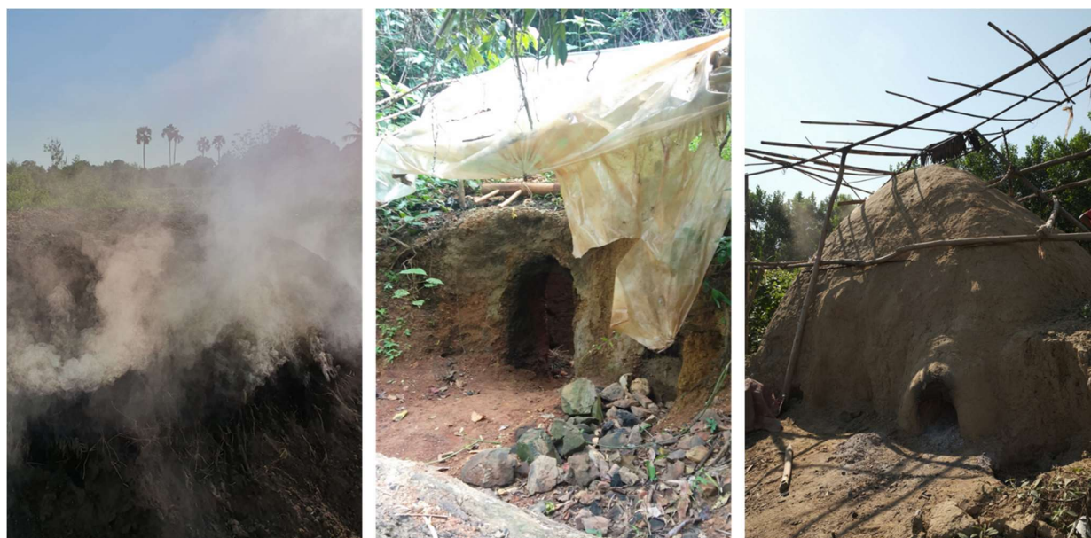
Figure 73 - Charcoal kilns of increasing technical sophistication
