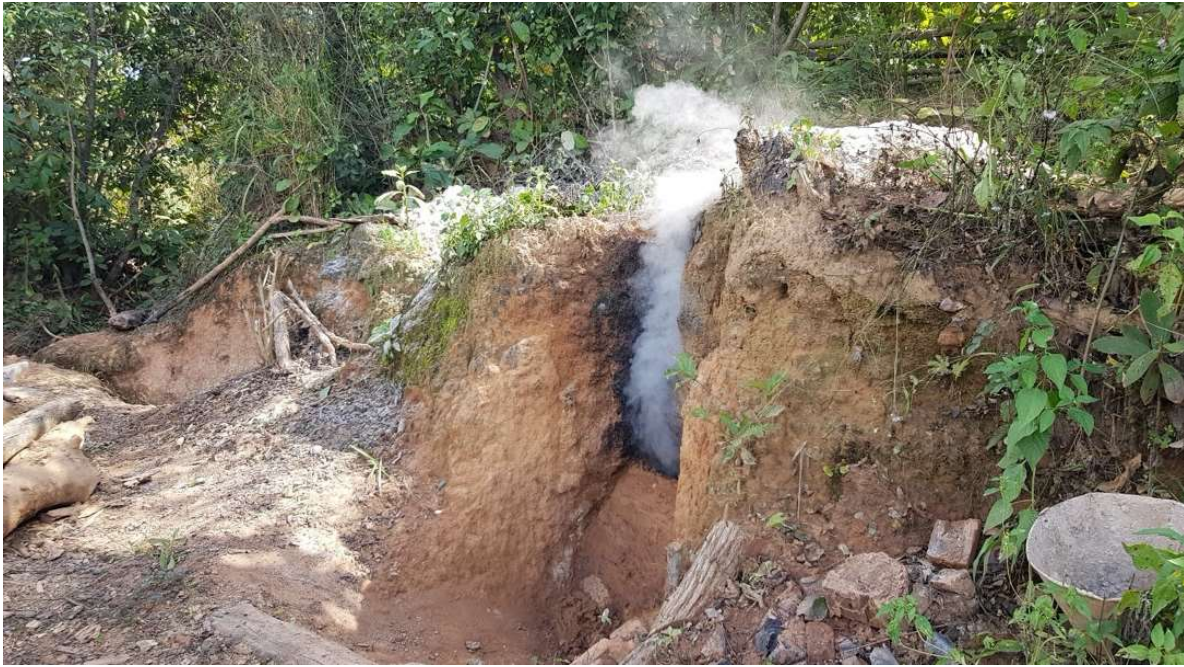
Figure 40 - Charcoal pit kiln in Mandalay Division
