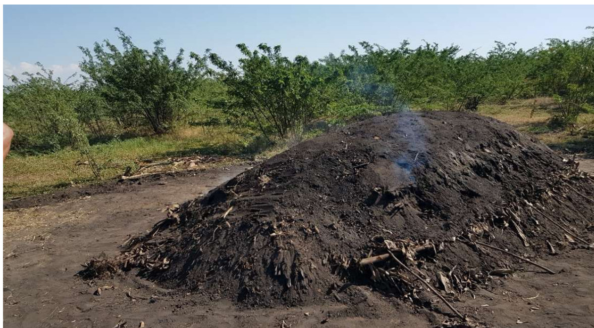
Figure 39 - Earth mound charcoal kiln in Mandalay Division
