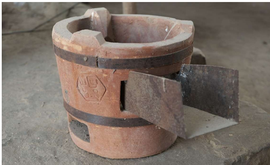
Figure 62 - A1 stove modified by Myanmar Biomass Power to be used with pellets
