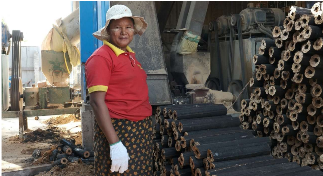
Figure 59 - Worker in a rice husk briquette and pellet factory in Sagaing division
