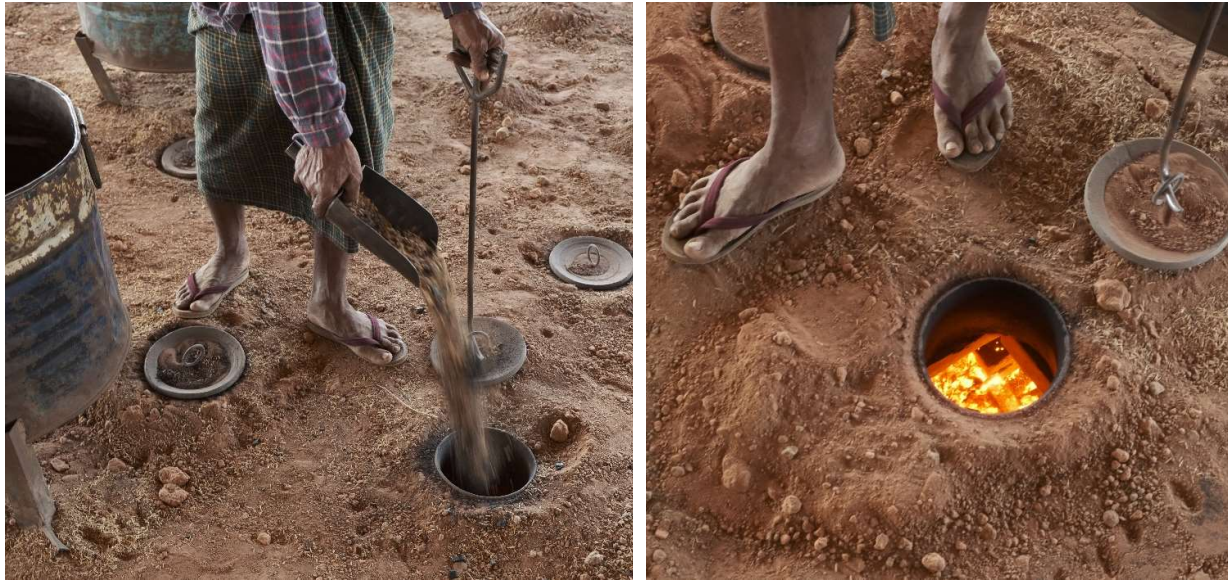
Figure 85 - Worker adding a mix of rice husk, sawdust, and coal to a Hoffman brick kiln in Mandalay
