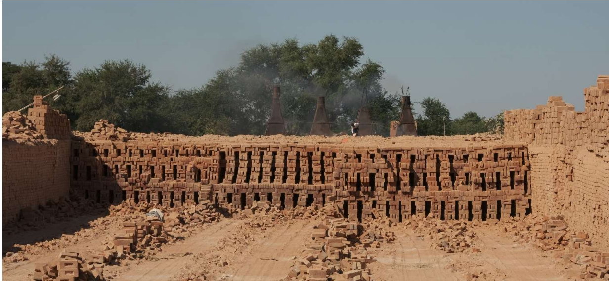
Figure 83 - Chimney Bull Trench Kiln using firewood, Mandalay Division
