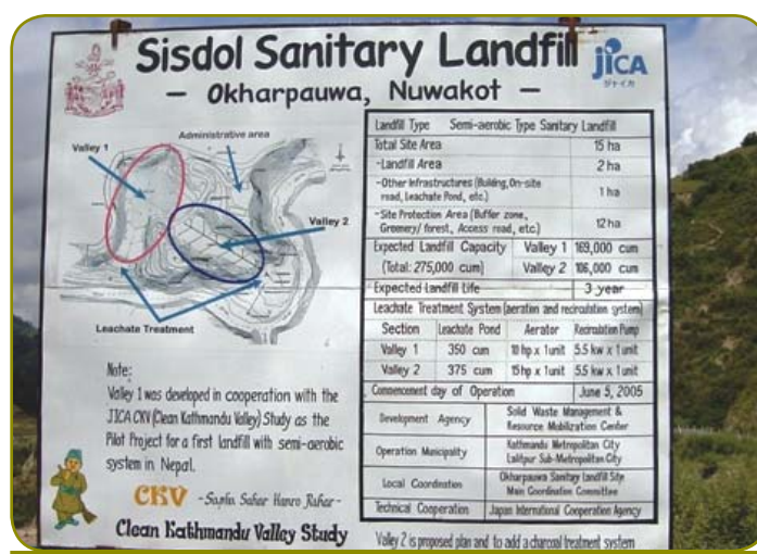
Sign at the entrance to Sisdol Sanitary Landfill in Nepal providing basic design details. Photo by Sumith Pilapitiya, Lead Environmental Specialist, South Asia Sustainable Development, The World Bank.
