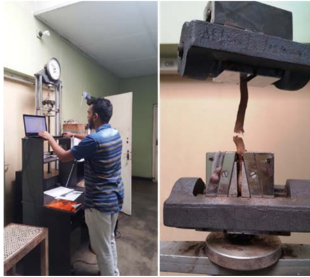
Figure 3-2 Root tensile strength testing using Dynamometer
