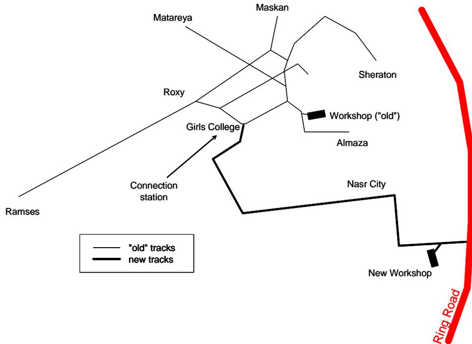
Sketch showing old tracks of tramway lines that will be converted into 3 BRT corridors, and the new tracks for the LRT and its extension to the Ring Road/New Cairo. Girls College station will be an intermodal connection station (Metro, BRT, LRT)
