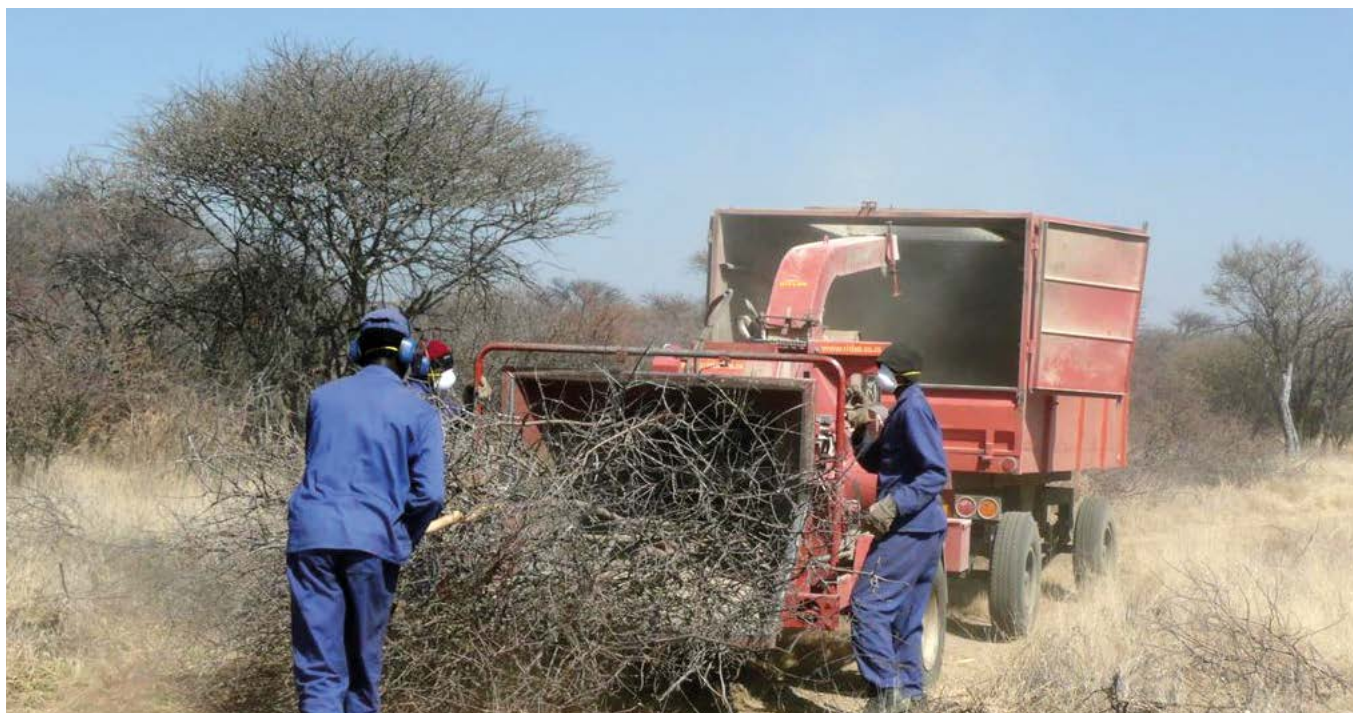
Manual bush harvesting with axes and mechanised processing into wood chips, Otjozondjupa Region Namibia (Cheetah Conservation Fund).
