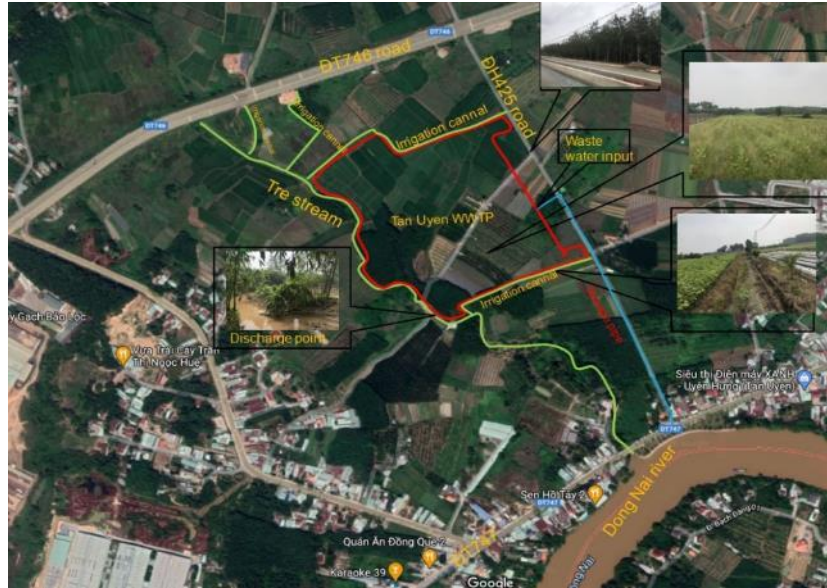
Figure 3.5. Location of the WWTP and surrounding objects.
