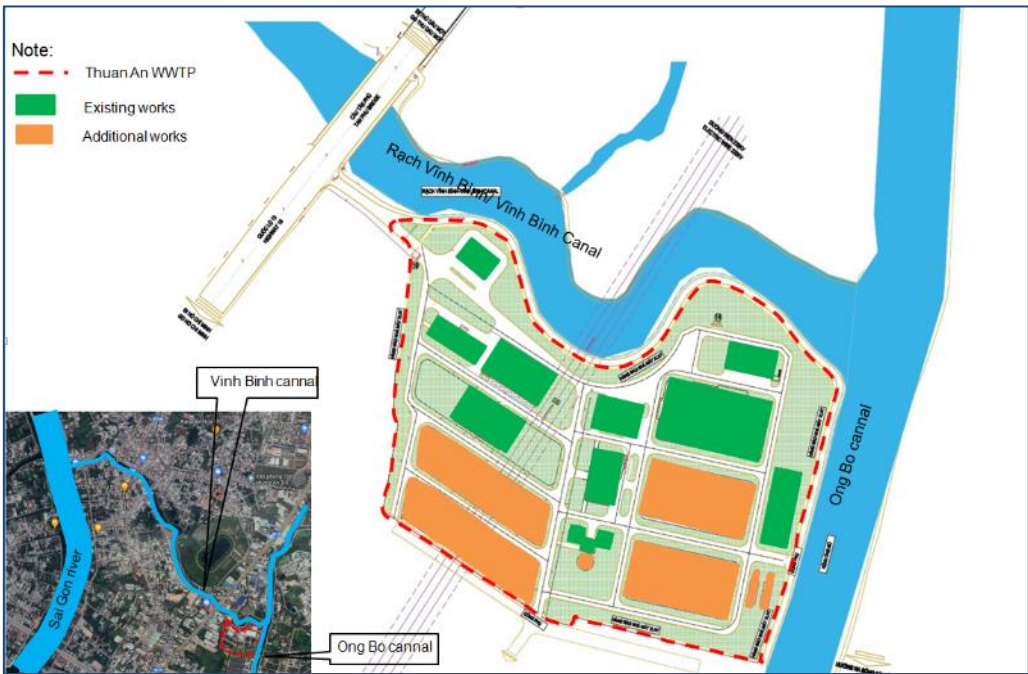
Figure 1.6. Layout of Thuan An WWTP.
