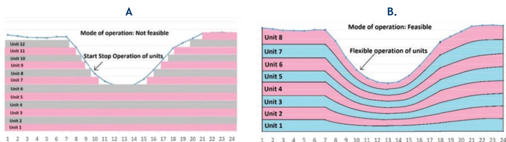
Figure 41: Mode of operation of thermal projects in the presence of large solar PV output
