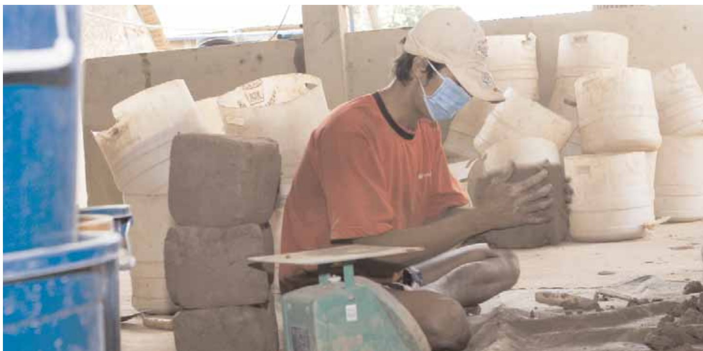
Blocks of clay (mixed with rice husk) are shaped and weighed before being pressed into the final pot shape
