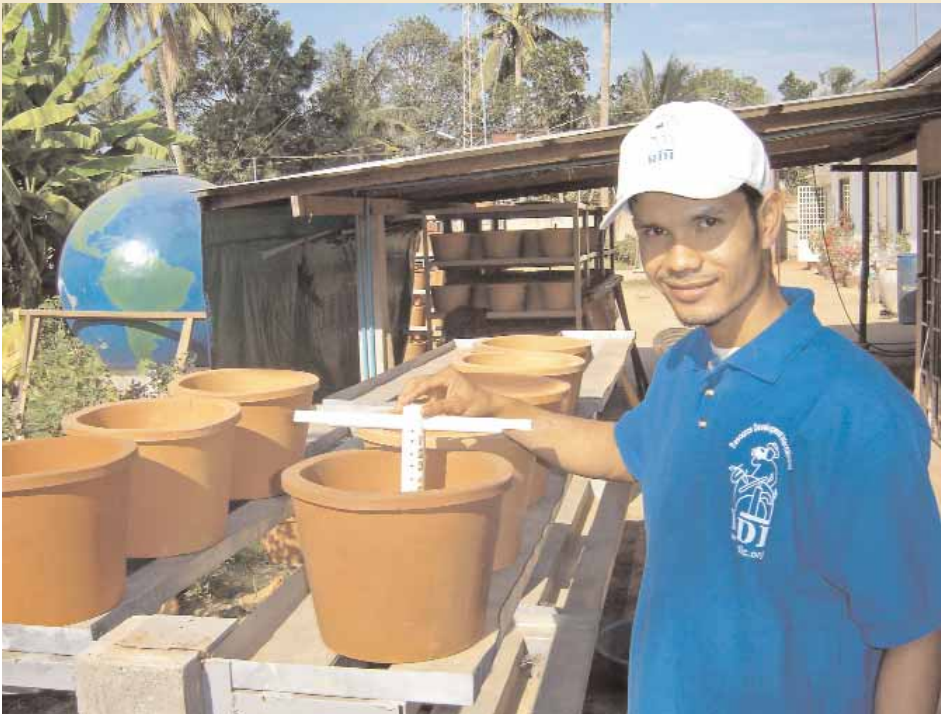
After firing the pots, making sure that the flow rate is within the acceptable range is an essential quality control step
