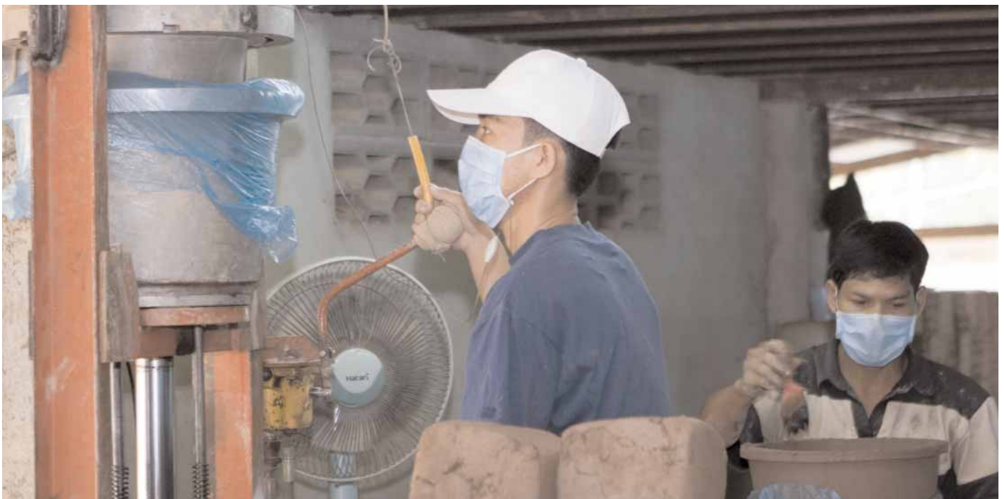
The pots are shaped by hydraulic press, operated by a skilled worker
